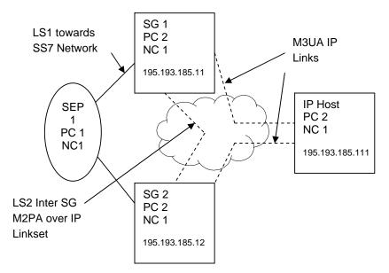
The following configuration commands are for SG1 and SG2, where SG1 and SG2 are in DUAL operation and SG1, SG2 and the IP host are acting as a single Point Code. Note the configuration of LS2 between the two SGs and the use of this link set for routes to the SS7 network.
